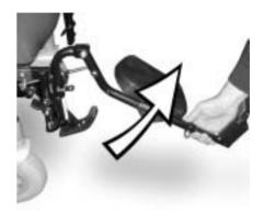
• To lower the legrest, press the lever (1) down and adjust the legrest to the desired position.
